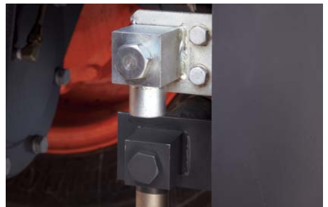
Engine oil and coolant drains Drains are installed in very accessible places to facilitate emptying without the risk of polluting the environment.
