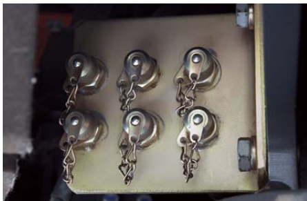
Hydraulic pressure check points The pressure test points are grouped together. (Main pressure, steering, braking etc).
