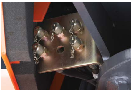
Hydraulic pressure check points The pressure test points are grouped together. (Main pressure, steering, braking etc).
