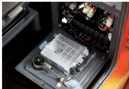
Transmission diagnostics The transmission and engine can be diagnosed using a laptop computer to interface with the diagnostic system.
