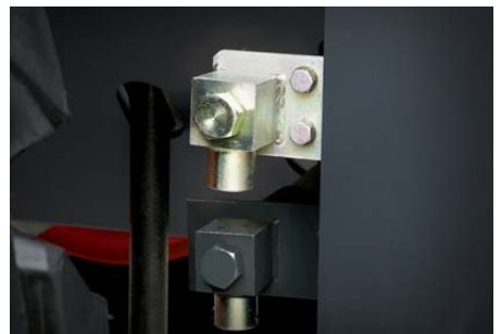
Engine oil and coolant drains Drains are installed in very accessible places to facilitate emptying without the risk of polluting the environment.
